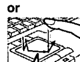
Two quick taps, but on the second tap leaving your finger down (applying pressure) and moving it on the work surface. One tap when your finger will "drop" the object.
